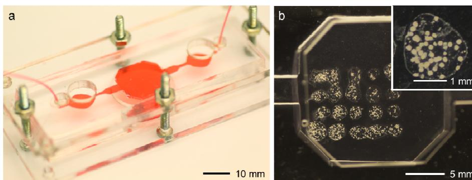
Figure 1. Liver-on-a-chip system: (a) 2 PMMA sheets, tightened by screws, hold the PDMS top layer and glass bottom layer together. (b) HepG2/C3A liver cells embedded in GelMA bioprinted on the microbioreactor.
